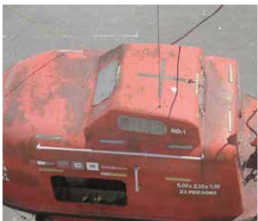
Poor condition of lifeboat hull.
